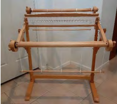
This is a Kromski rigid heddle loom with a 24" weaving width looking from front to back.
