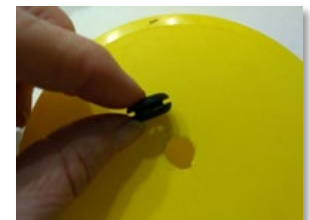
Use a grommet in the lid for a tighter fit
