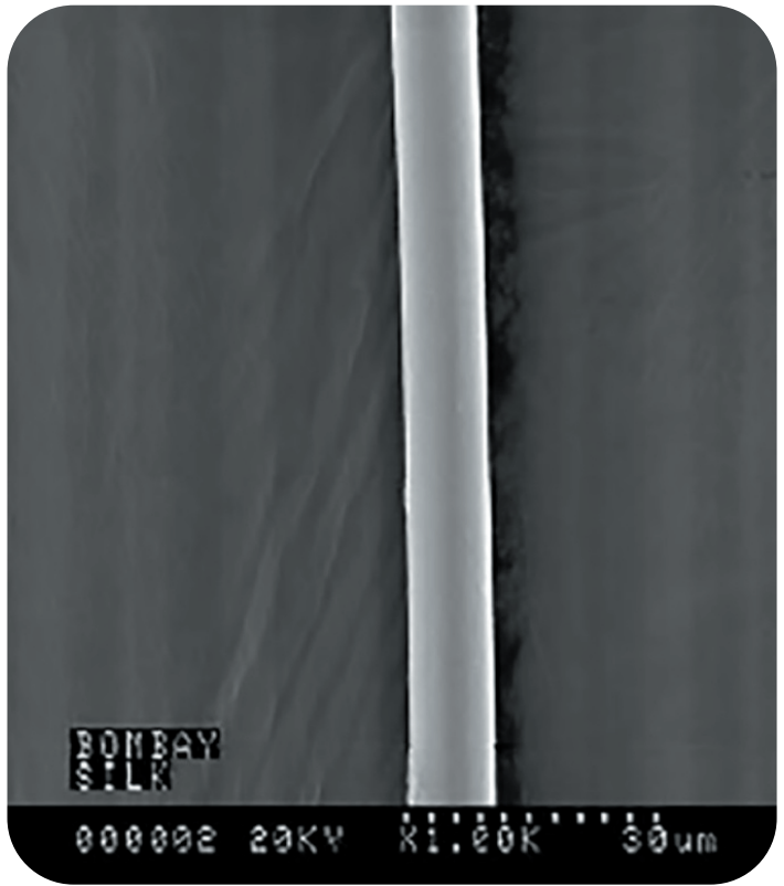
Bombay Silk -AFD 10-12 microns. Silk does not have a cuticle scale since it is reeled together from 4-20 filament ends from the silk worm.
